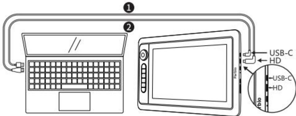
Figure 2-1 Connection Method 1
