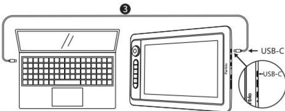
Figure 2-2 Connection Method 2
